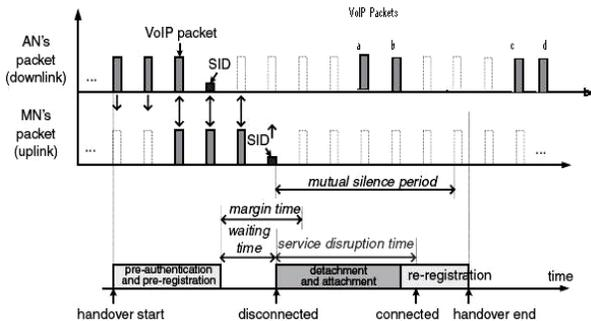
Figure 2: Breaking of silence before completing VHO
